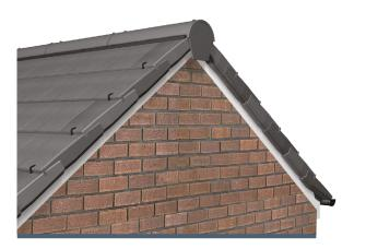
Fix Battens and underlay in accordance with BS 5534. Insert the Verge Units before fully fixing the battens into place. Underlay should extend 10mm beyond the outer face of the gable structure. Battens must be cut inboard of the outer face of the gable structure by no more than 15mm (Picture 1).
