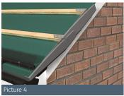
For stone verge pack only - apply a verge foam to the inside edge of each unit to close off the gap between the verge unit and the uneven wall surface.
