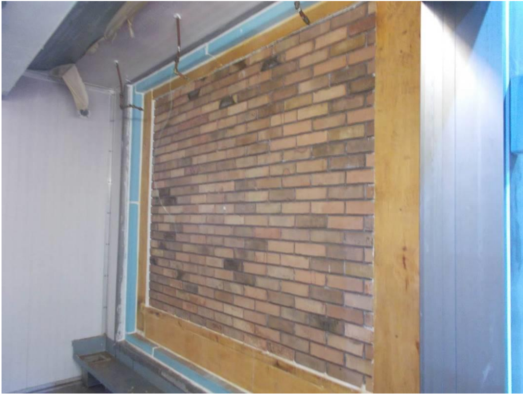
Plate 3 - Face of Panel Prior to Test
