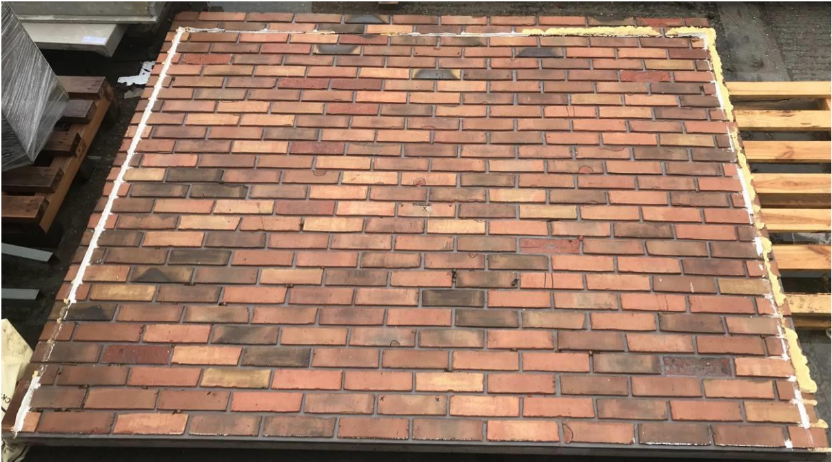
Plate 7 - Panel after Impact and Bond Strength Testing
