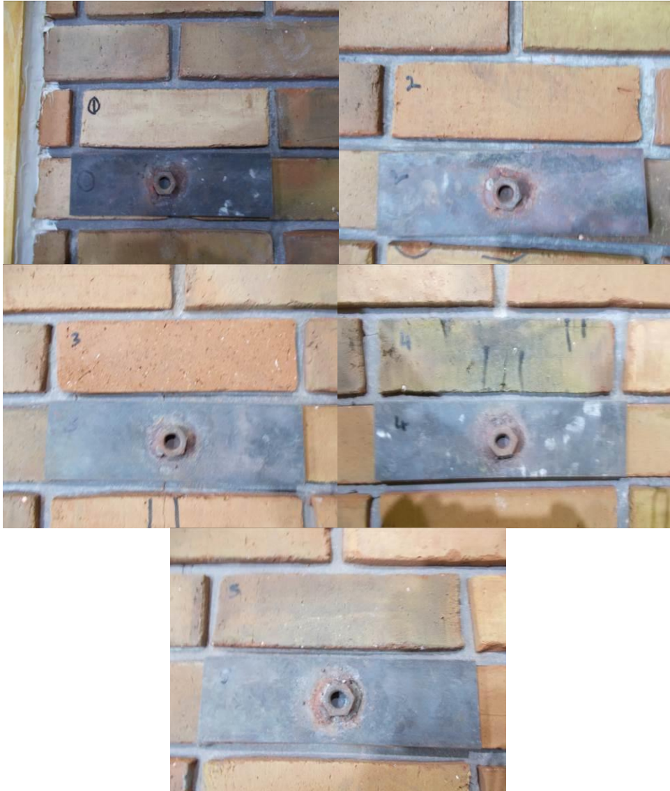
Plate 1 - Typical Failure Modes Bond Strength
