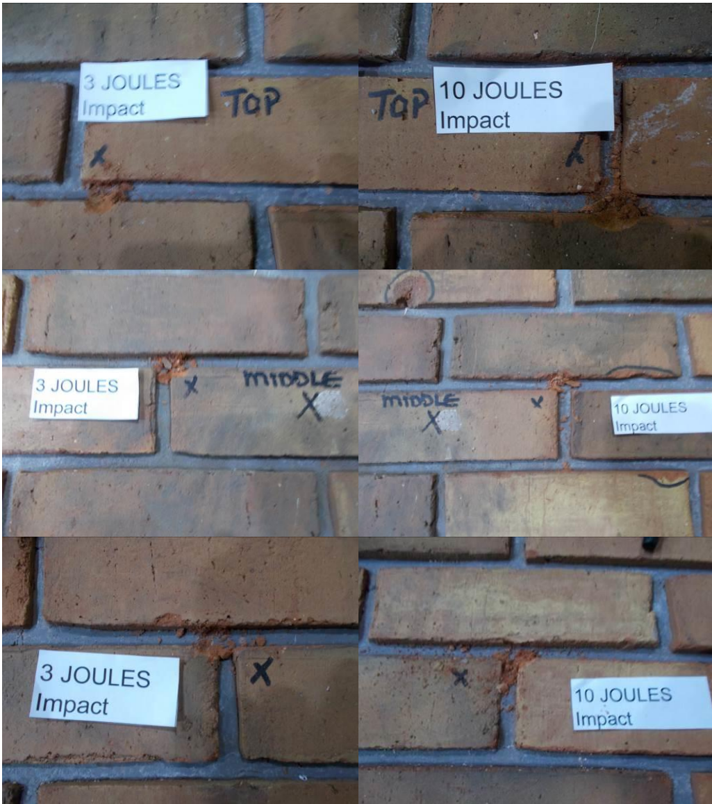
Plate 2 - Typical Damage Hard Body Impact Testing
