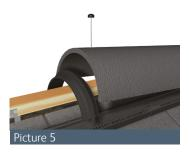
7) Continue fixing nailhole ridge tiles, top fillers and ridge seals along the ridge. If cutting is necessary to maintain the aesthetics of the ridge line, the block end ridge must not be cut. Ridge tiles must not be cut to less than half of their original length. All ridge tiles must be twice fixed with drive screws supplied (re-drill nailholes if necessary). At the verge, trim the last top fillers and fix the block end ridge tile as described in step 6 to finish the ridge line (Picture 6).
