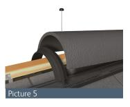
7) Continue fixing nailhole ridge tiles, top fillers and ridge seals along the ridge. If cutting is necessary to maintain the aesthetics of the ridge line, the block end ridge must not be cut. Ridge tiles must not be cut to less than half of their original length. All ridge tiles must be twice fixed with fixings supplied (re-drill nailholes if necessary). At the verge, trim the last top fillers and fix the block end ridge tile as described in step 6 to finish the ridge line (Picture 6).
