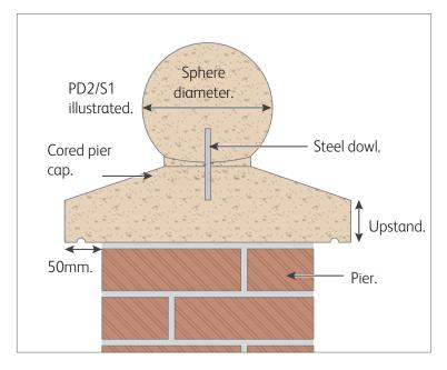
The sphere aperture must be filled with masonry epoxy adhesive and the dowel inserted and hardened before placement.
