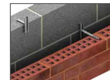
TWO PART TIES, ADJUSTABLE UP OR DOWN VIA A CHANNEL FIXED TO THE BLOCKWORK
