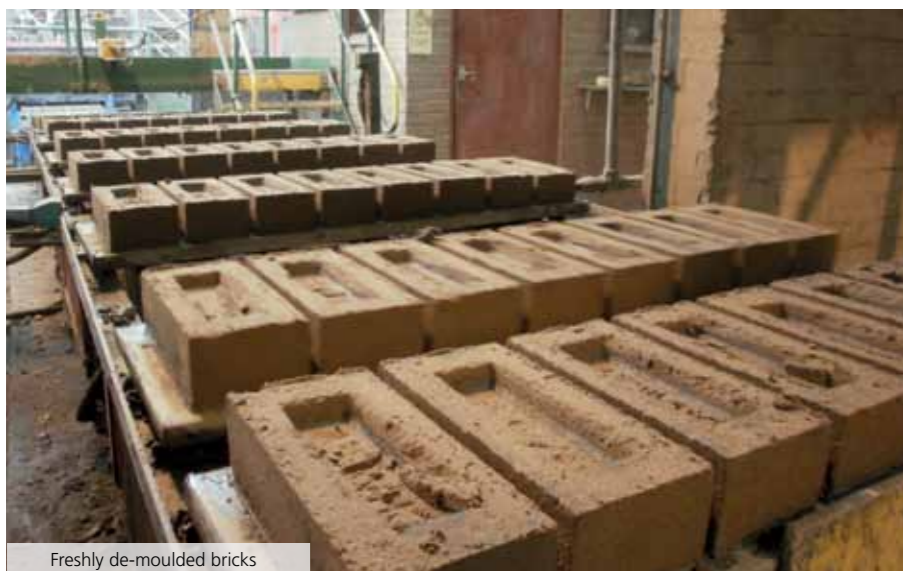
Freshly de-moulded bricks
