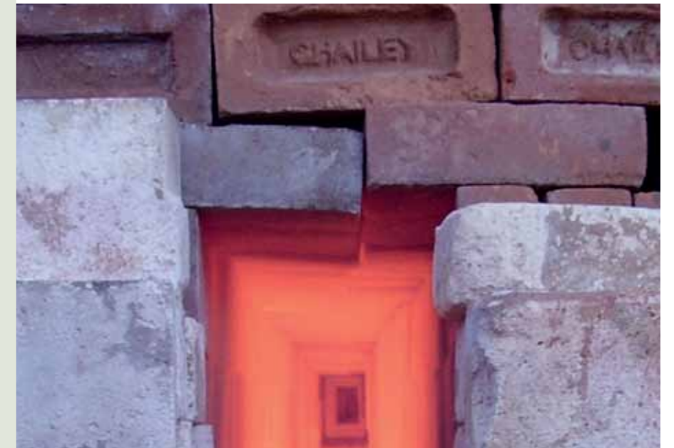
A view down a fire hole into the heart of the clamp (where the temperature can reach in excess of 1050°C.)
