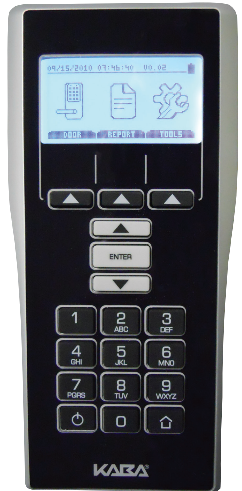
Kaba's M-Unit is a user-friendly portable programming and auditing device.
