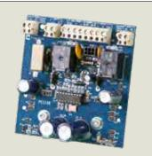
The Keyscan DPS-15 is a dual-linear DC power supply with two outputs for ACU-12VDC at 1.2 Amperes and AUX/RDR-12VDC at 1.2 Amperes.
