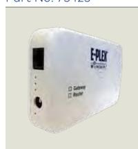
An E-Plex Gateway provides two-way communication from an E-Plex Lock to Keyscan Aurora software. A Gateway communicates to Aurora by a direct connection to a USB (non-network) or TCP/IP network. A Router acts as a repeater, extending the radio frequency (RF) communication between the Gateway and E-Plex Locks.
