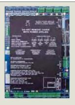
The Keyscan CA4500B is a access control panel only. It is available to replace non-functioning CA4500 access control panels.
