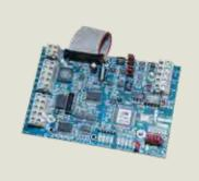
A new communication control module designed to use a CAN Bus communication network. The CIM provides optimized server to Access Control Unit (ACU) communication giving users an ACU to ACU network providing inter-panel communication for global functions. The CIM also includes enhanced device-based diagnostics and improved communication speeds.
