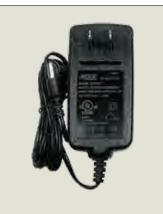
The PS1225 is a replacement 12VDC plug-in switching transformer for the SDACSKT (SDAC Kit). Plugs into standard 120 Vac outlet and provides up to 2.5 amps. Has 60" of 18 Gauge cable for mounting close to SDAC control. Has 2.1 mm barrel power connector. Center positive. For replacement of transformer provided in the SDACSKT. C/UL/US Listed Black Colour
