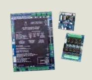
The Keyscan CA4500NBM is a network appliance-based access control unit that gives you unmatched flexibility for new installations or revitalizing aged or failing access control systems. The CA4500NBM is a package that includes 1 CA4500B ACU board, 1-OCB8 relay board, and 1-DPS-15 power supply. This hardware is programmed for up to 90,000 credentials. This does not include a black metal enclosure.
