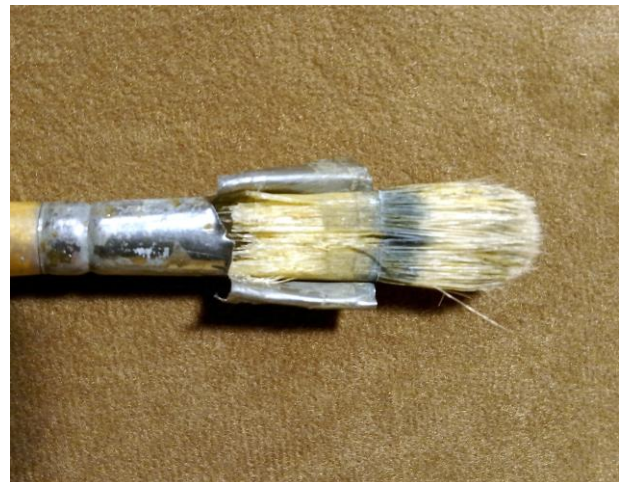
Well-worn brush with ferrule cut away, revealing full bristle length
