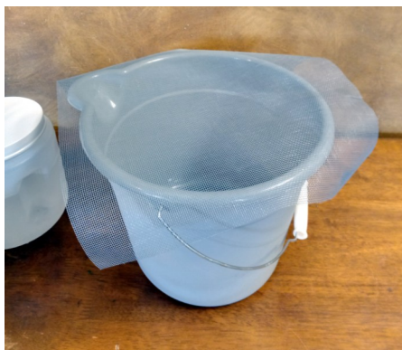
Small plastic bucket covered with screen, used for evaporating paint waste water
