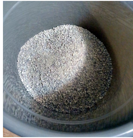
Cat litter placed in the collection bucket to displace and absorb standing liquid
