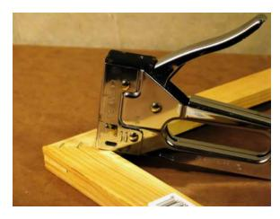
To keep corners in square without a glue bond, insert several staples across each joint. Staples should be removed before displaying finished art.
