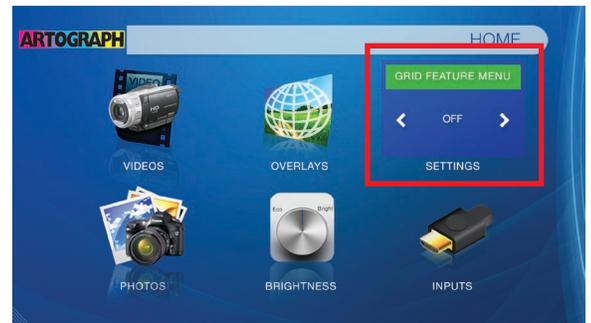
To dismiss the dialog box after selecting the desired grid, press the “return” button on the remote or the top of the projector. Alternatively, you can access the grids BEFORE you select an image by selecting the “OVERLAYS” icon in the main menu.
