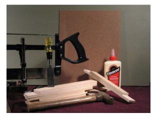
Select clean, knot-free pine boards for bracing. Tools include a saw, hammer and wood chisel, sanding block and file.
