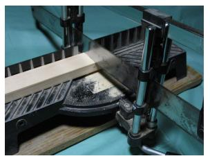
Cut across the board at 90 degrees, half the height of the brace.
