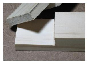
Lap joints offer good surface area and resist diagonal distortion.
