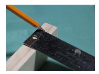
Cut braces the same dimensions as the panel. Measure to cut lap joints on each end, parallel line half the height of the board, and perpendicular (cross cut) equal to the width of the board.
