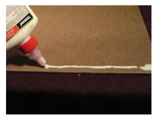
Place panel face down on a clean surface. Apply glue on all four sides.
