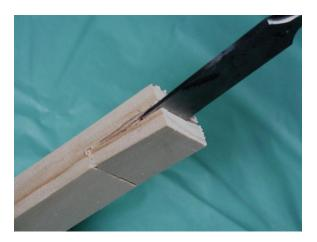
Use a sharp chisel to remove excess wood. If necessary, clean up with a file or sanding block to achieve a flat, square joint.
