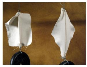
Note that the length of stretch possible on the bias is significantly greater. By displacing the weave rather than trying to elongate the yarns, greater length is achieved and, on a stretcher chassis, tension is distributed more uniformly across the fabric.
