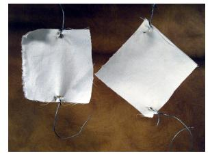
The samples were weighted: one in the direction of the warp yarns and the other diagonally across the weave.
