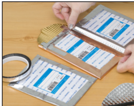
Step 5: Using metallic tape, attach panels to form a triptych.
