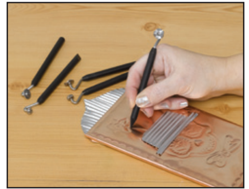
Step 2: Emboss tooling foil with various tools.
