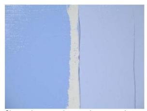
Observe the contrast between the two samples. The sample with better dispersed, more heavily pigmented paint will exhibit a greater degree of color change, and will appear more intense and dark. Firmly scrape down the bottom half of each sample to reveal undertone.
