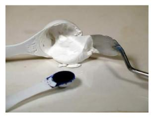
Place the white paint on the glass palette along with the first sample of color. Use a palette knife to remove as much paint as possible from each spoon.
