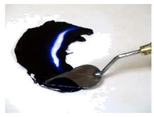
Spread the sample thinly on the palette, noting viscosity. Gather with the putty knife and observe how well the paint forms and retains peaks; note any slumping of the pile.
