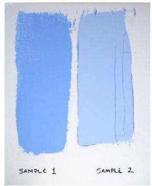
When a homogeneous mixture has been achieved, use the putty knife to place a stripe of sample #2 on the canvas board, as close as possible to the first without mixing or touching.
