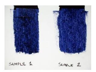
To reveal undertone, perform a draw-down, using the putty knife to create a stripe of color on a canvas board. Firmly scrape down the bottom half of the sample so the canvas is visible. This technique is also useful to reveal a difference in covering power between two test colors.
