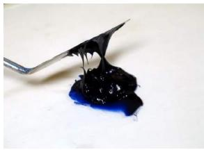
Press down with a palette knife and lift. Note the "length" of the sample, whether it pulls in strings or breaks short.
