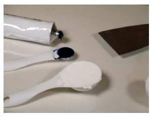
Measure one level ¼ teaspoon of each color and two level tablespoons of the standard white. Take care to eliminate any air pockets in the measuring spoon. Select sample #1 and one spoon of white; set aside sample #2 and the remaining white.
