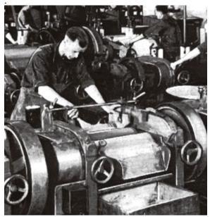
The Roller Mill is one of the powerful machines we use to make many of the products artists use every day. Making paint involves much more than simply mixing pigment with a vehicle. Milling brings out the peak intensity, luminosity and covering power of pigments. Properly milled paint is stable and workable, totally consistent from batch to batch.
