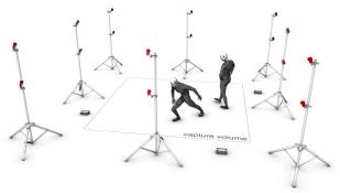
Cameras should be placed around the capture volume so that the markers will be within view of at least two cameras at all times. Aim cameras so that the maximum overlap of camera view occurs in the region where most of the capture will be taking place. For more information, visit the Arena tutorials:
