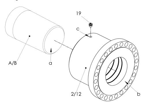
Fig. 6-2 Mounting the hub with conical oil interference fit
