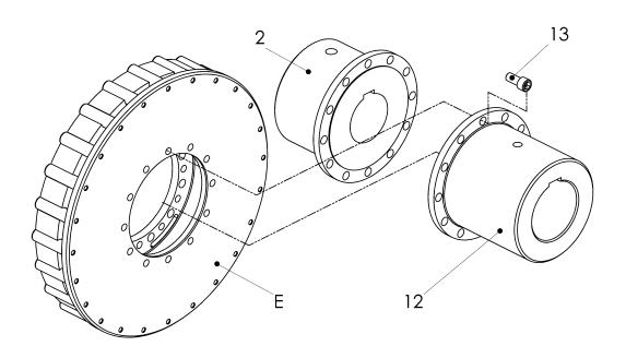
Fig. 6-6 Mounting the pre-mounted adapter with rubber element (E)
