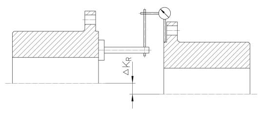
Fig. 5-2 Radial misalignment
