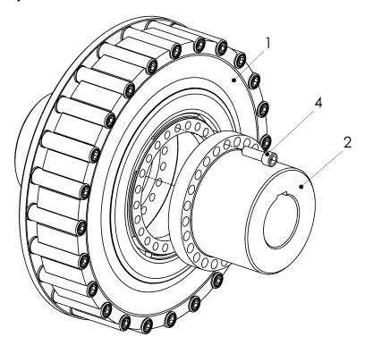
Fig. 6-7 Mounting the rubber element (coupling sizes 0800...4000 and 8000...18000
