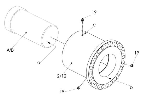
Fig. 6-3 Mounting the hub with cylindrical oil interference fit
