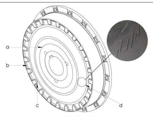
Fig. 8-1 Visual inspection at the rubber elements
