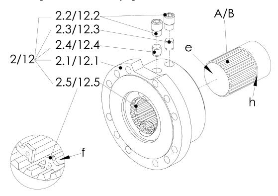
Fig. 6-4 Mounting the CENTALOC clamping hub
