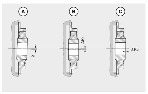
The permissible coupling misalignment limits are dependent on multiple factors such as e.g. coupling size, element hardness, operating speed and torque stress. The guideline values listed in the following table apply to a medium element hardness and a typical rotational speed up to 1500 rpm<sup>-1</sup>.
