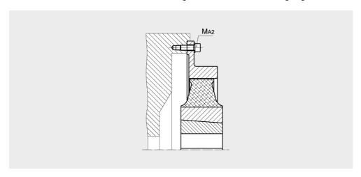
▶ Before tightening the bolts make sure that the washers have full-surface contact on the flange.
