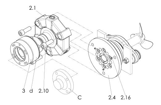
Fig. 6-11 Mounting the Homokinet to the rubber element
