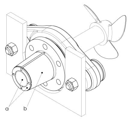
Fig. 6-5 Propeller shaft and bush are flush before mounting
