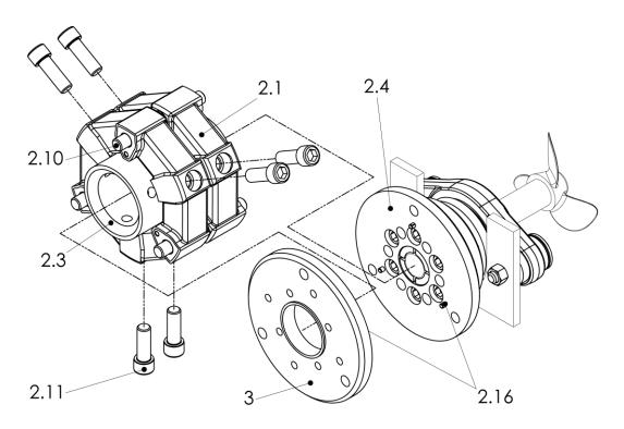
Fig. 6-10 Mounting the set with the rubber element
