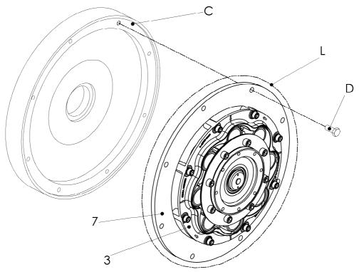
Fig. 6-2 Mounting the coupling with adapter to the flywheel
