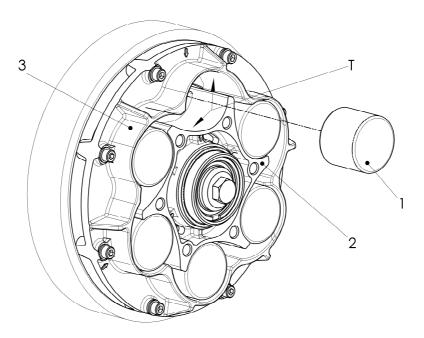
Fig. 8-2 Dismantling the rubber rollers
