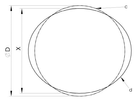
Fig. 8-3 Oval deformation of the rubber roller
