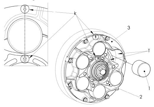
Fig. 8-4 Reassembling the rubber rollers
