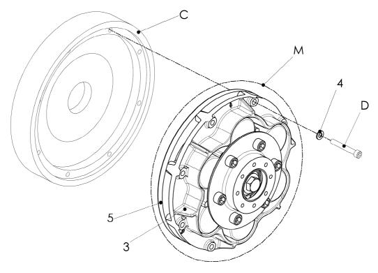
Fig. 6-1 Mounting the coupling to the flywheel
