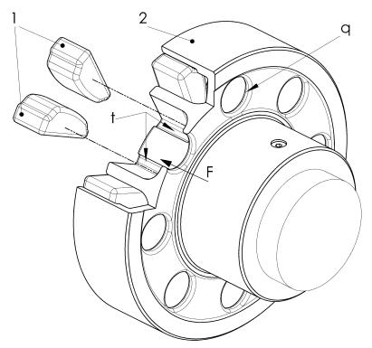
Fig. 9-1 Replacing the rubber elements (1)
