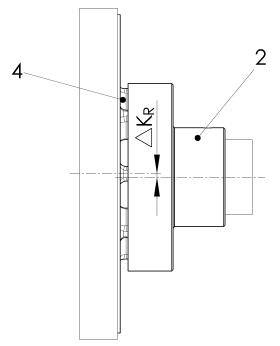
Fig. 5-2 Radial misalignment
