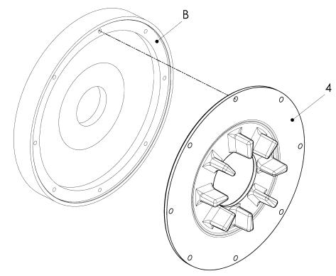
Fig. 6-5 Mounting the inner part (4)
