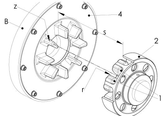
Fig. 6-6 Connecting the driving and driven units
