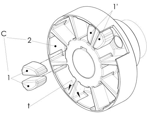
Fig. 6-4 Mounting the rubber elements
