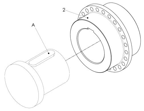
Fig. 6-1 Mounting the hub with cylindrical bore and keyway
