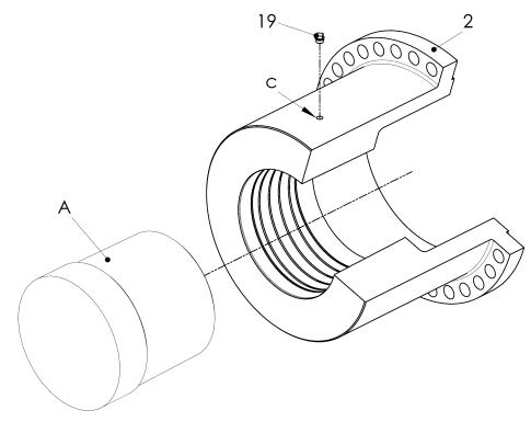
Fig. 6-2 Mounting the hub with conical oil interference fit
