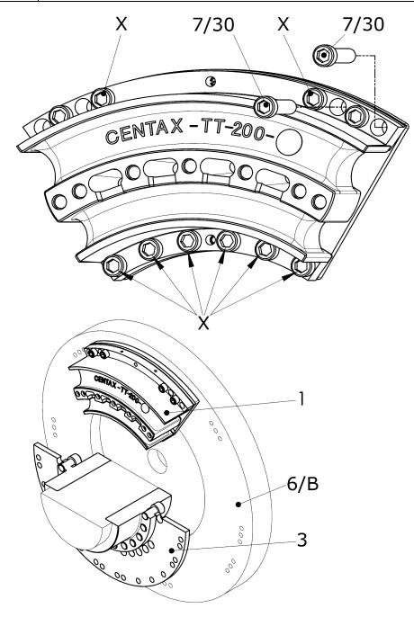
*Fig.* 6-9 *Mounting the rubber elements of coupling size 200*
