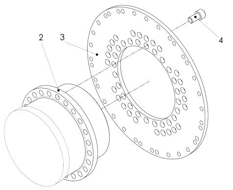
Fig. 6-4 Mounting the adapter of coupling size 130-360
