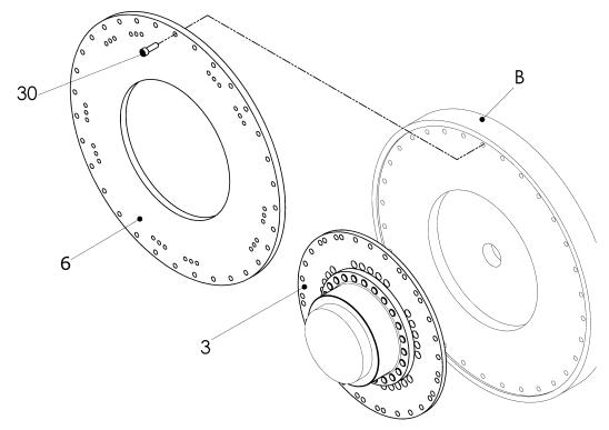
*Fig.* 6-6 *Positioning the adapter* (6) *to the flywheel (type FS)*
