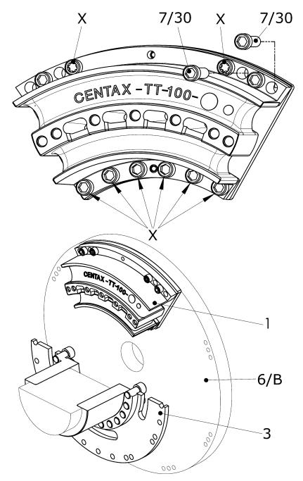
Fig. 6-8 Mounting the rubber elements of coupling size 100
