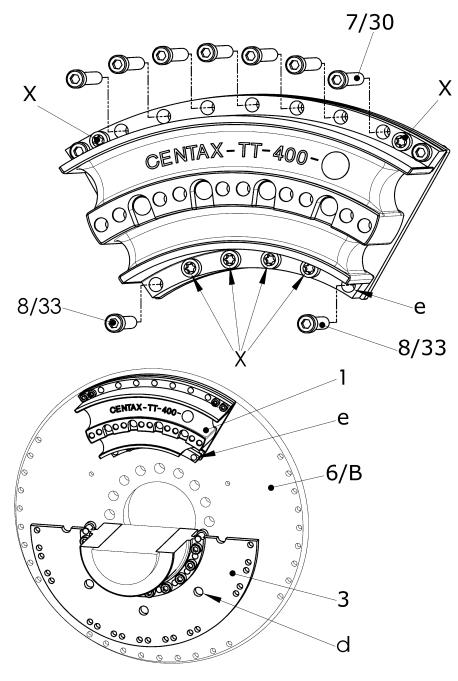
*Fig.* 6-11 Mounting the rubber elements of coupling size 400
