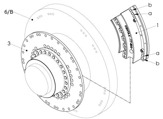
*Fig.* 6-7 *Positioning the rubber elements*
