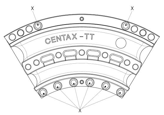
Fig. 9-3 Precompressed rubber element size 100-200
