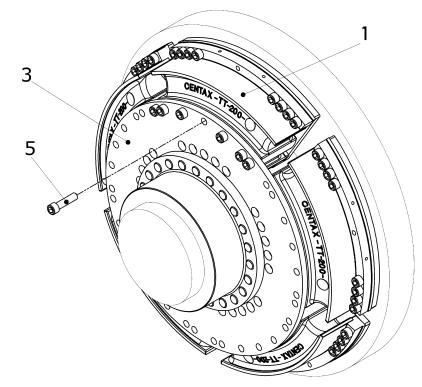
Fig. 6-13 Mounting the adapter (3) to the rubber element
