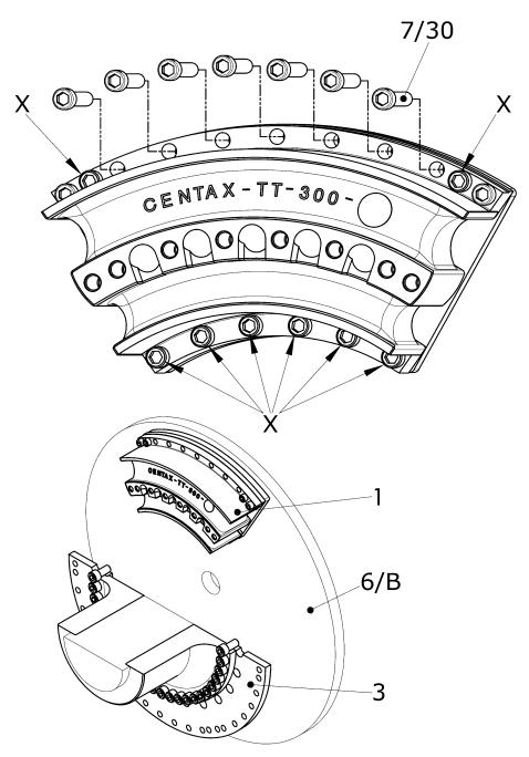
*Fig.* 6-10 Mounting the rubber elements of coupling size 300
