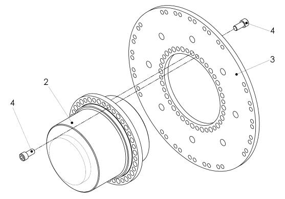
Fig. 6-5 Mounting the adapter of coupling size 440-460
