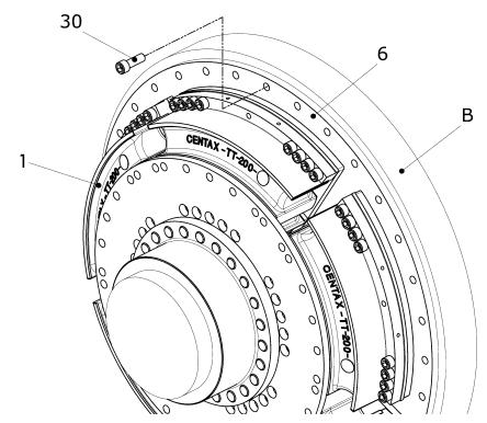
Fig. 6-12 Mounting the adapter to the flywheel (type FS)
