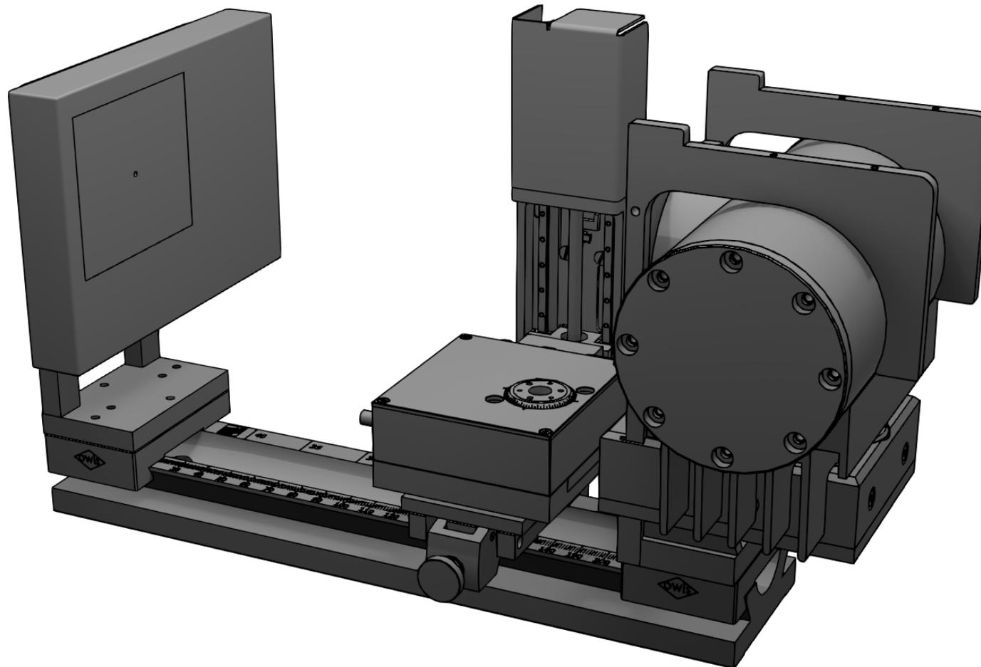
Concept drawing showing the inside of the CT-PORTABLE. This system is extremely versatile due to its size and light weight.
