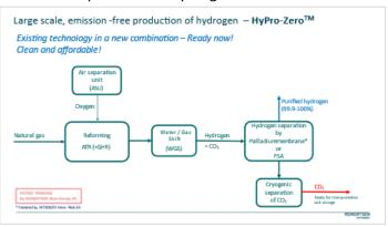
The process solution has been further developed to an ultrahigh CO2 capture rate of close to 100% and no need for import of renewable electricity. The technology is proven and can be built, now! Ready now!
