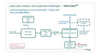
The hydrogen production cost, including CCS is estimated to 1.5 - 2.0Euro/kgH2, the higher figure is valid for ultra-high CO2 capture rate and no power import. The production cost of blue hydrogen is less than half of green hydrogen!
