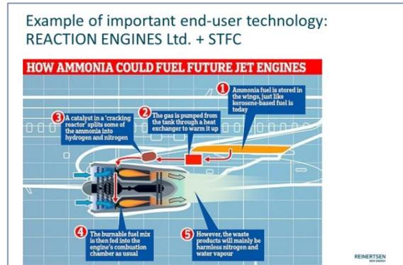
Ammonia is to be stored in the aircraft as regular airfuel. Part of it will have to be cracked to hydrogen. The mixture is fed to the jet engines. The heat required for the cracking comes from the exhaust.
