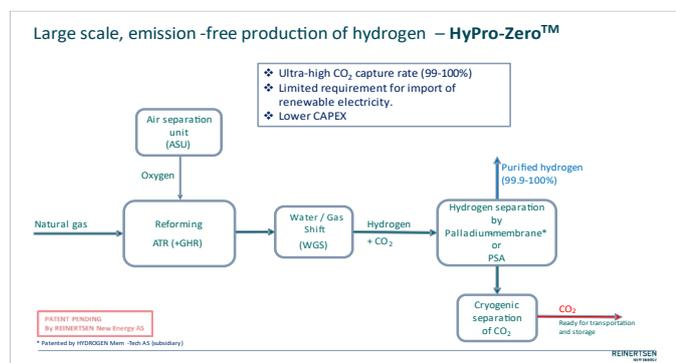
Clean ammonia may also be efficiently produced based hydrogen production processes like the HyPro-Zero™. The bi-product, nitrogen from the ASU is combined with clean hydrogen in the production of ammonia.
