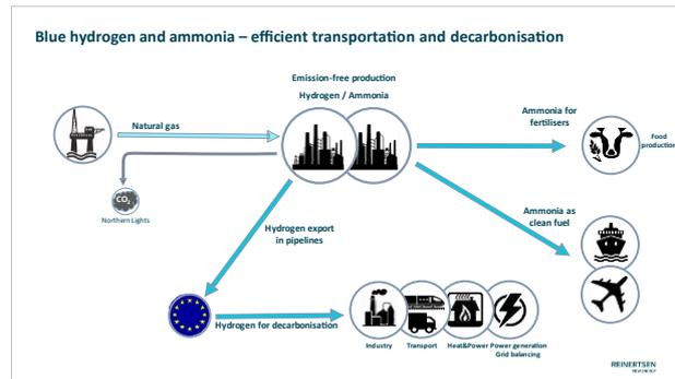
The current, end user technology developments include 100% hydrogen and 100% ammonia as fuel for turbines and internal combustion engines (ICE). As fuel cells are very limited in capacity, the development of turbines and ICEs are important for power generation, compression, marine shipping and possibly aviation (jet engines).
