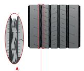
Tapered sinusoidal grooves facilitate additional reinforcement on continuous channelized ribs therefore enhancing vehicle stability.
