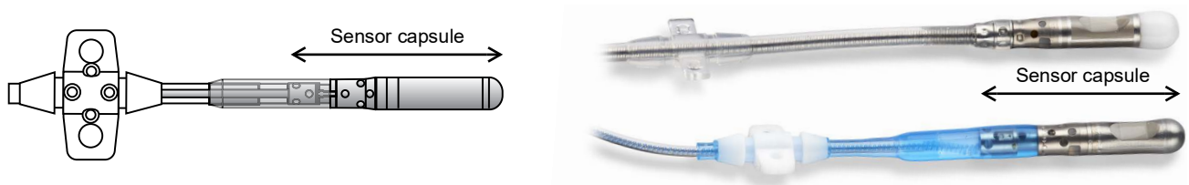
Figure 4. Images of the sensor capsule on the distal end of the sensing lead
