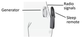
Figure 4. Communication between sleep remote and generator
