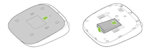
Warning! Device must be powered off before installing or replacing the nano-SIM card.
