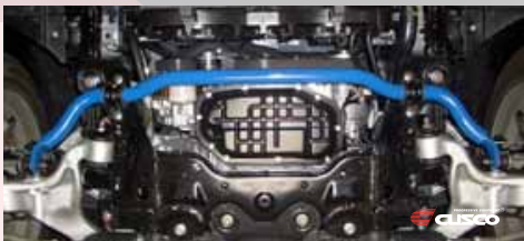
J50 2WD FRONT SWAY BAR PART NO: 252 311 A28 MSRP: $374 USD HOLLOW 28mm 119% EFFECTIVE
