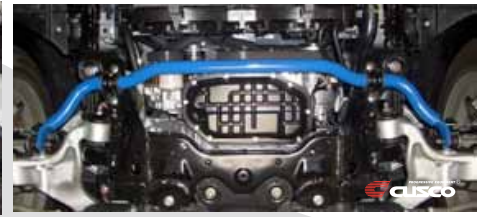
NJ50 4WD FRONT SWAY BAR PART NO: 257 311 A35 MSRP: $440 USD HOLLOW 35mm 120% EFFECTIVE
