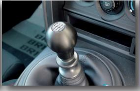
44mm OD shift knob made to fit the palm of your hand perfectly with FR-S shift pattern, Duracon material. The height of this shift knob is made exclusive for this application to enable factory feel when engaging the reverse ring.
