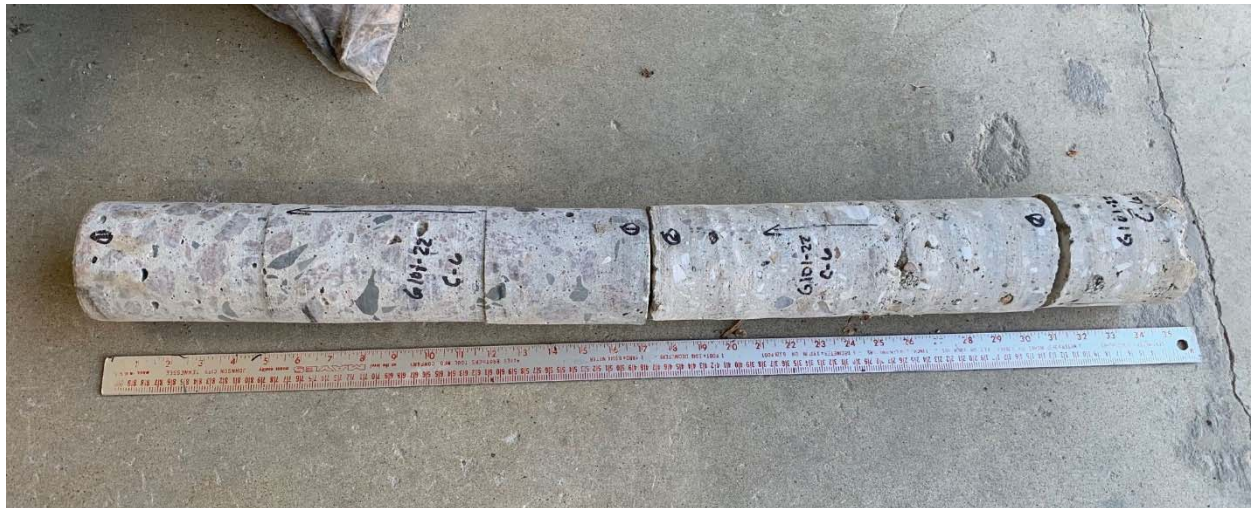
Photo 2 - Core C-6, 16.75" concrete, 16.5 cement-treated base
