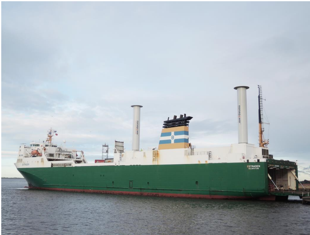
Bore's Ro-Ro vessel MS Estraden with two Norsepower Rotor Sails installed onboard.
