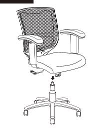
Now turn the assembled seat upright and locate the center hole of the Mechanism over the Seat Post. Push down firmly until the connection is secure.
