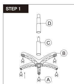
Press the Casters (A) into the holes at the end of each leg of the Base (B).
