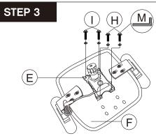
Please be careful to use the correct RED Mechanism Rear Screws and Washers (H) and BLUE Mechanism Front Screws and Washers (I).
