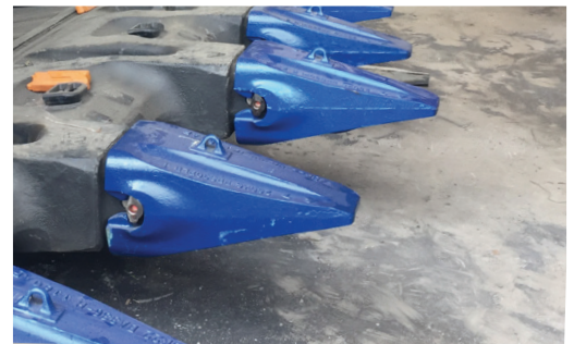
PPS30PLB Solid Point at installation
