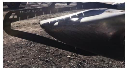
Gauging of Position 1 point at final inspection and removal
