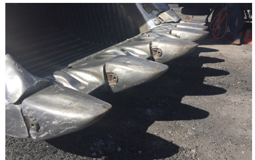
Solid points at final inspection and removal
