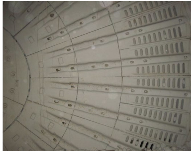
Figure 6 – Radial Discharge End Grate Design
