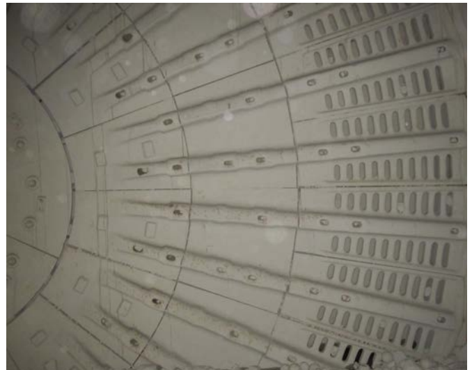
Image 4 – Radial Discharge End Grate Design
