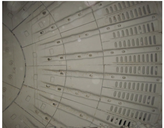
Image 4 – Radial Discharge End Grate Design
