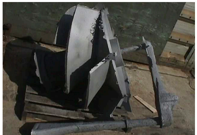
Figure 4 – 2,600 lbs. open impeller made in a three-part mould. Alloy: CF-3M
