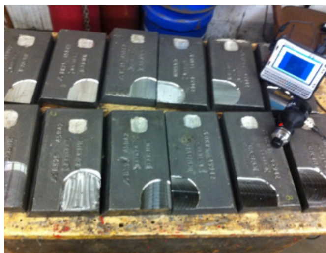
Figure 1 – Cast weld test plates
