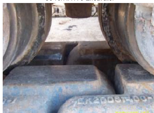
Bradken's patented continuous roller path
