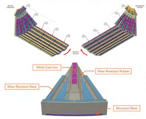
Rubber composite liners with high resistance laminated steel inserts (500 to 550 HB) and high chrome cast inserts (650 HB) have demonstrated longer wear life and uniform wear than CrMo castings in high abrasion grinding.
