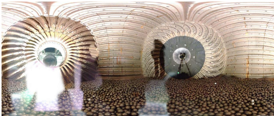
Figure 19 – The New Stage 1 Liner Designed Installed in April 2018
