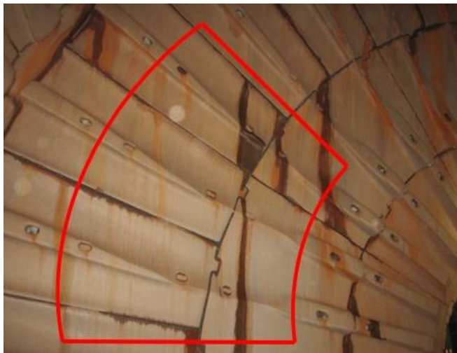
Figure 5 – Feed End Liners showing High Wear Zone
