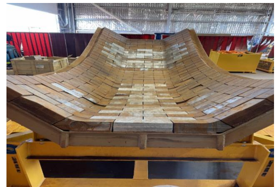
New blocks of the high wear area kit (silver/as cast) installed in the refurbished
