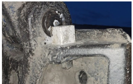
Bradken's upgraded pin retention hardware
