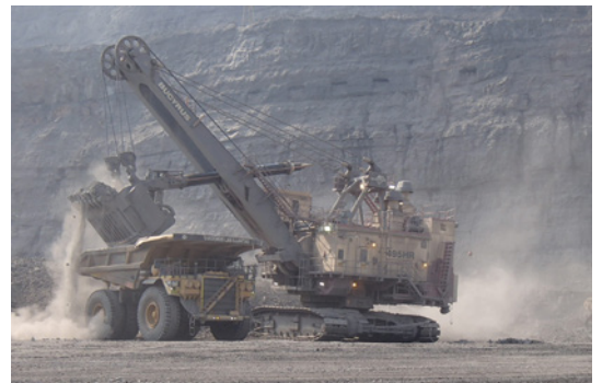
Bradken undercarriage on CAT7495 Excavator
