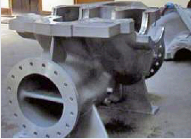
Figure 1a – Pump Casing Bottom
