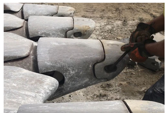
Eclipse Points are easily removed
